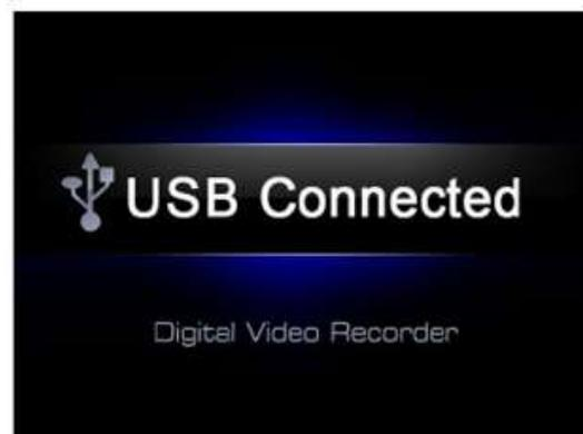
**Important Note:** When connected to a PC via USB all features **will not work** directly from camera, such as Record, Playback and Browse. Charging the battery will occur as well as data transfer via the connecting computer only.
