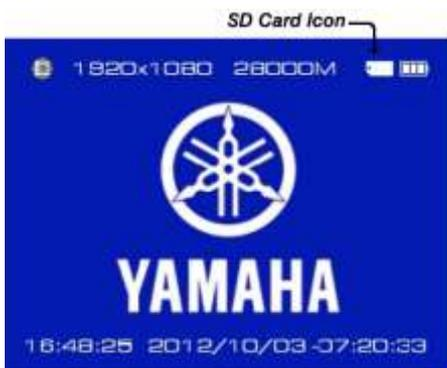
After installing the SD card, power on the camera and an SD card icon will appear in the top right corner of the screen – this indicates SD card is correctly installed. If no icon is displayed then an SD card is not installed or the card is invalid.
